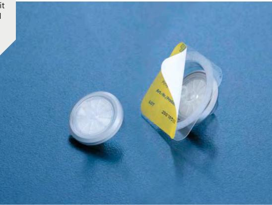
TPP syringe filters are intended to filter aqueous solutions such as tissue culture medium, buffers, protein solution, virus suspensions and DNA.
