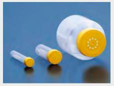
Filter screw caps for sterile gas exchange
