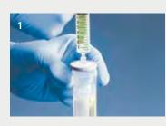
1. Stable fit of the filter on a 50 ml centrifuge tube
