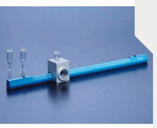
The PCV tube enables a quick and reproducible measuring technique of the cell volume. This quick method is ideal to monitor cell growth (cell mass).
