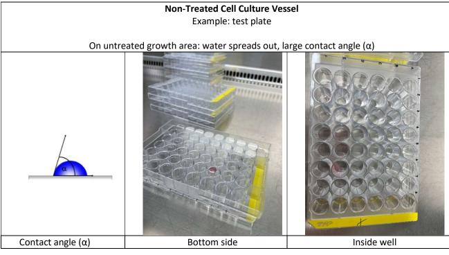
**Conclusion:** A simple and quick test to check for the presence of surface treatment in a vessel.
